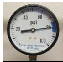
Inlet Gauge Peaks Between 75-85 psi
