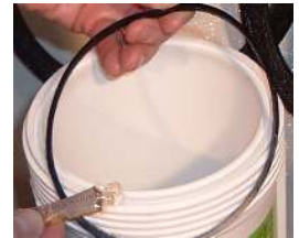
Replace each sump o-ring and lubricate with supplied lubricant.
